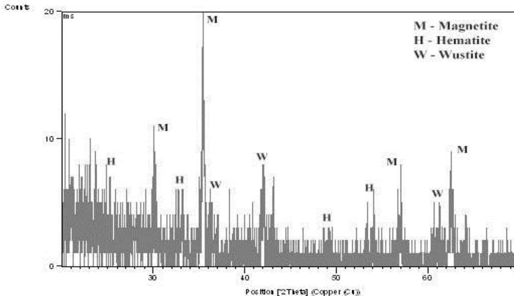
Figure 3. X-Ray Diffraction analysis of raw mill scale
