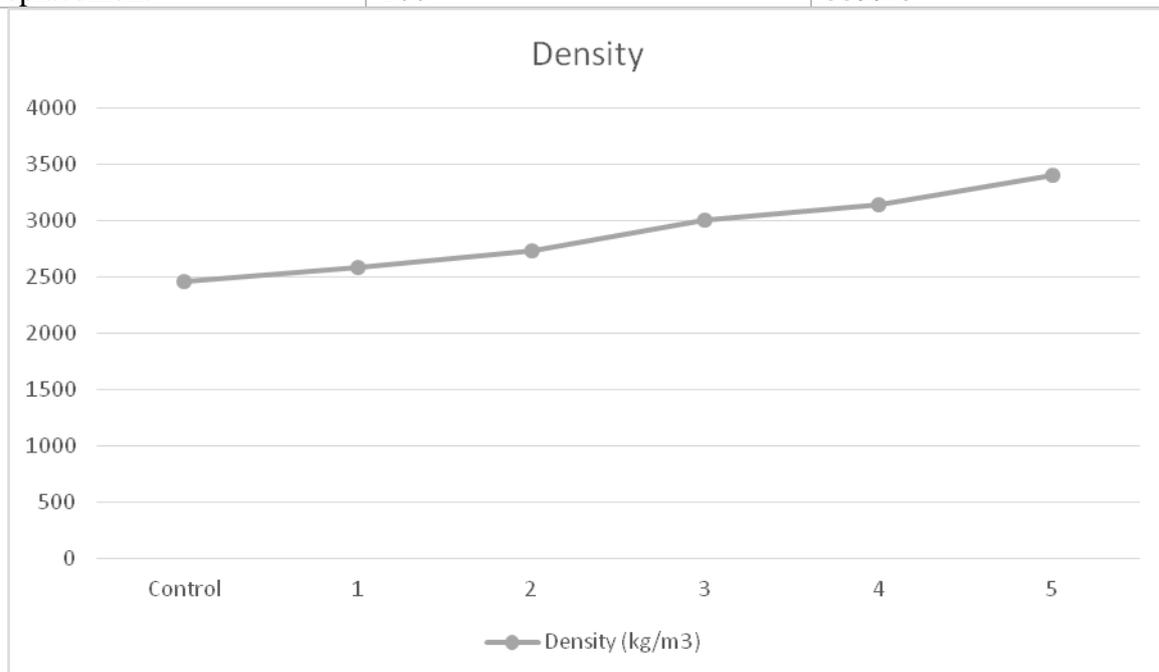
**Figure 4. Curve showing variation of density of different mortar samples**
