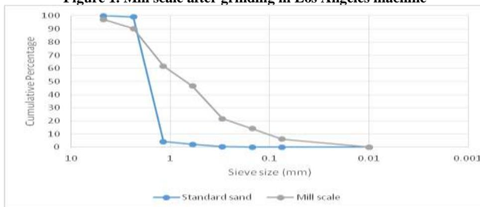
**Figure 2. Particle size distribution curve for mill scale and standard sand**
