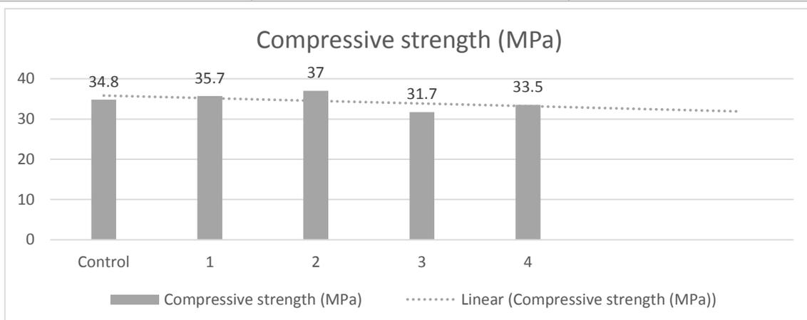
**Figure 7. Graph showing compressive strength of concrete samples after 28 days curing**
