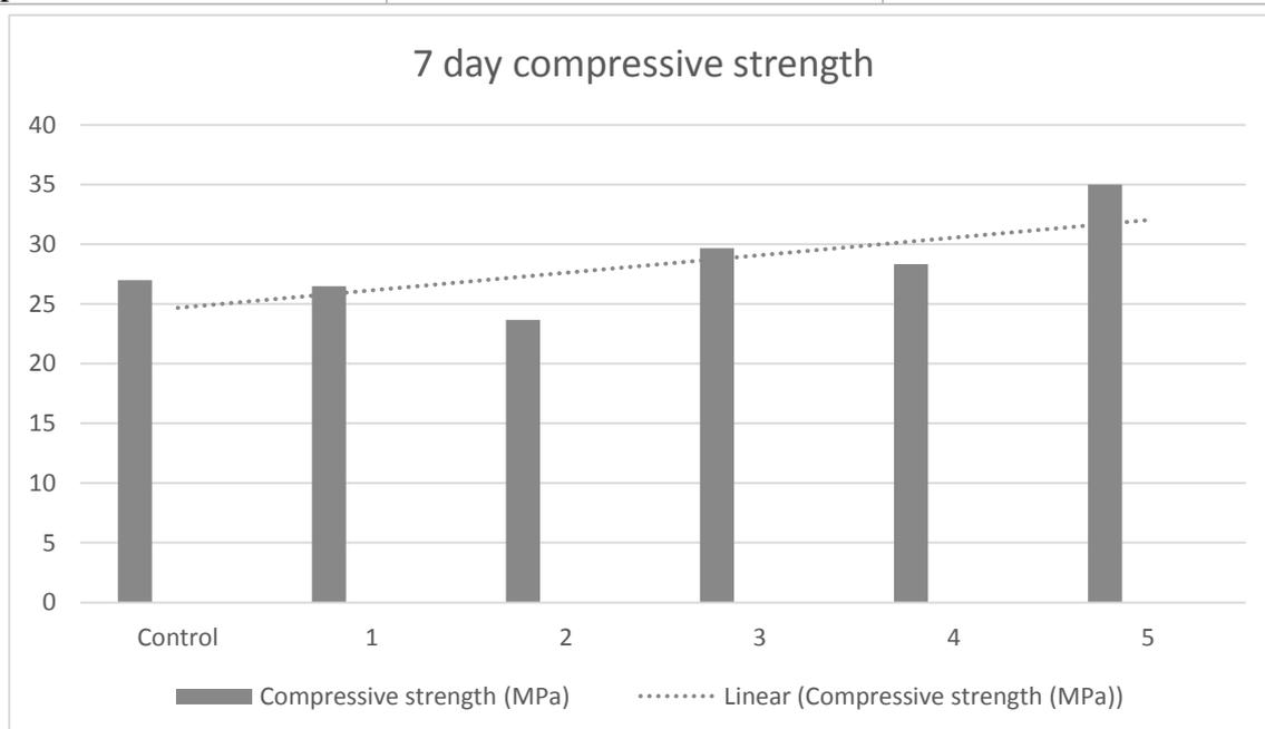
**Figure 5. Graph showing compressive strength of mortar samples after 7 days curing**
