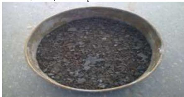
**Figure 1. Mill scale after grinding in Los Angeles machine**
