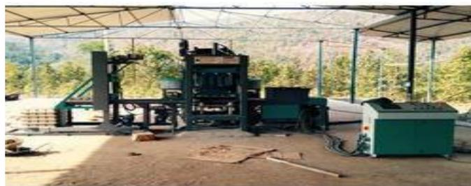
**Figure:- 1.2 Brick Moulding Machine**
