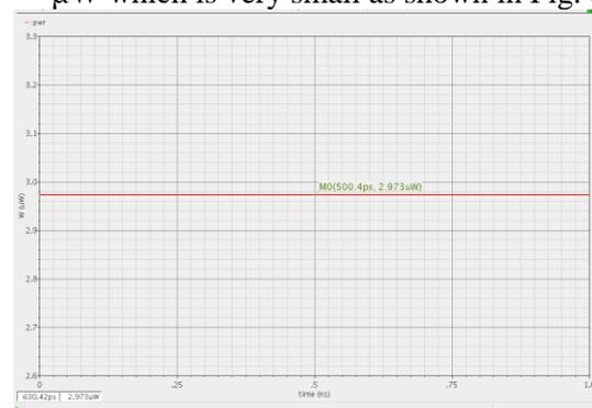
Fig. 7: Power dissipation of ring oscillator
