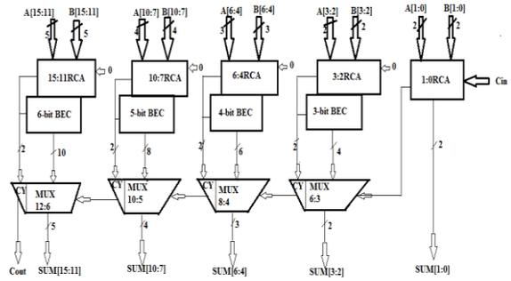
**Fig 3: Full adder using BEC**
