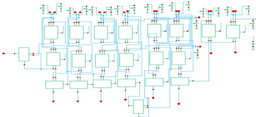
**Fig 5: Full adder with Transmission Gate**
