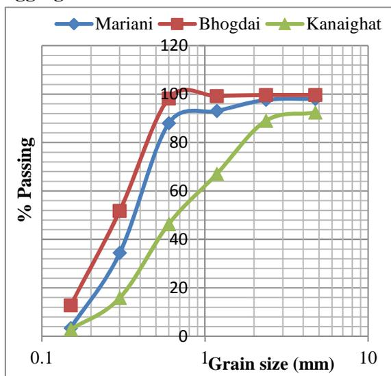
**Graph 2. Comparison of the sieve analysis of the 3 fine aggregates**
