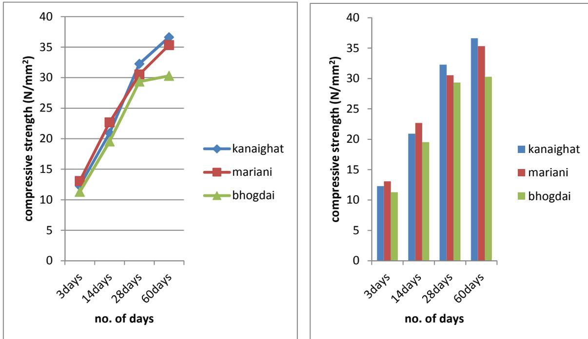
**Graph 4. Comparison of compressive strength of the cubes at the end of 28 days of curing and the target strength**
