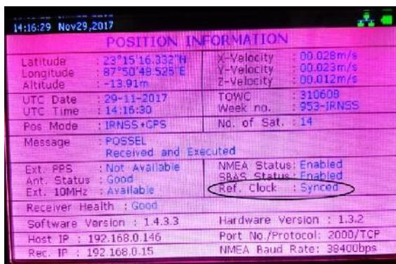
Fig. 2(a): Screenshot of the IGS receiver display panel after synchronization
