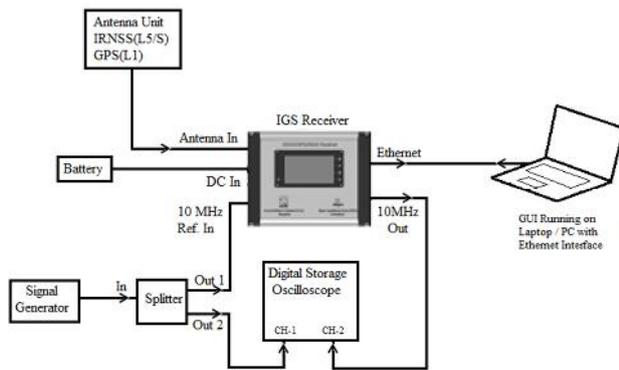
Fig. 1(a): Schematic of the experimental set up
