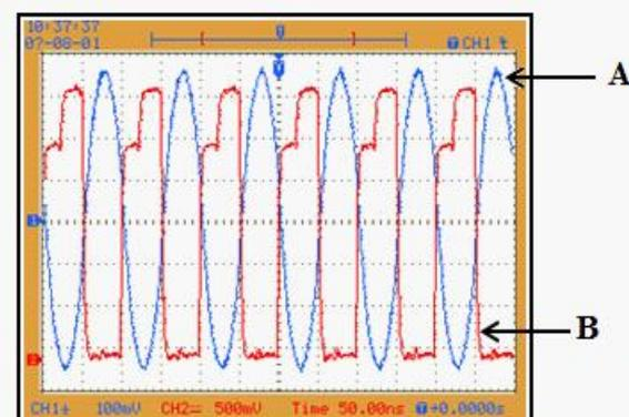
Fig. 2(b): Screenshot from DSO showing the input (trace A) and output (trace B) 10 MHz signal to the IGS receiver after synchronization
