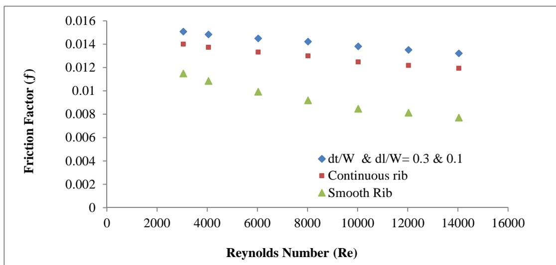
Figure (7) Variation of Friction factor with Reynolds number.
