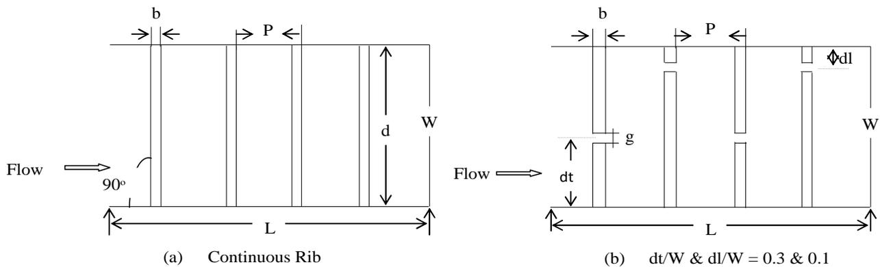
Fig.3. (a,b) Variation of with and without gap position at angle of attack ( ) 90° in a inclined ribs with a gap in staggered arrangements.
