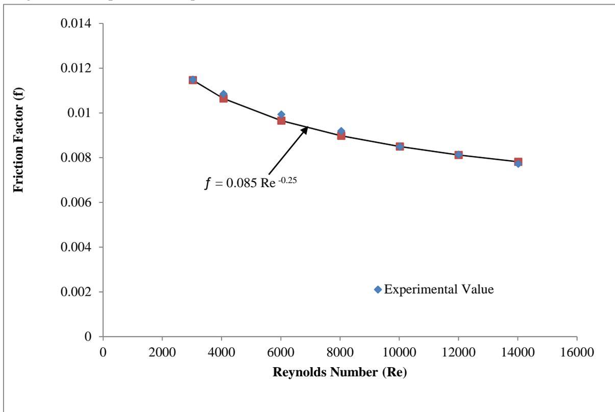
Figure (5) Comparison of experimental and estimated values of friction factor of smooth duct.
