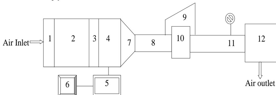
(1) Inlet Section, (2) Test Section, (3) Mixing Section, (4) Exit Section, (5) Data Tracker, (6) Computer, (7) Transition Section, (8) G.I. Pipe, (9) Inclined U-Tube Manometer, (10) Orifice Meter, (11) Control Valve, (12) Blower.
