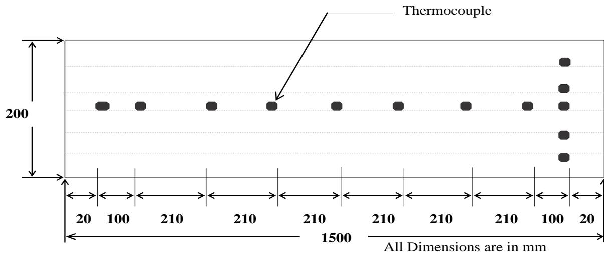
Fig.2. Position of thermocouples on absorbing plate (Test length).
