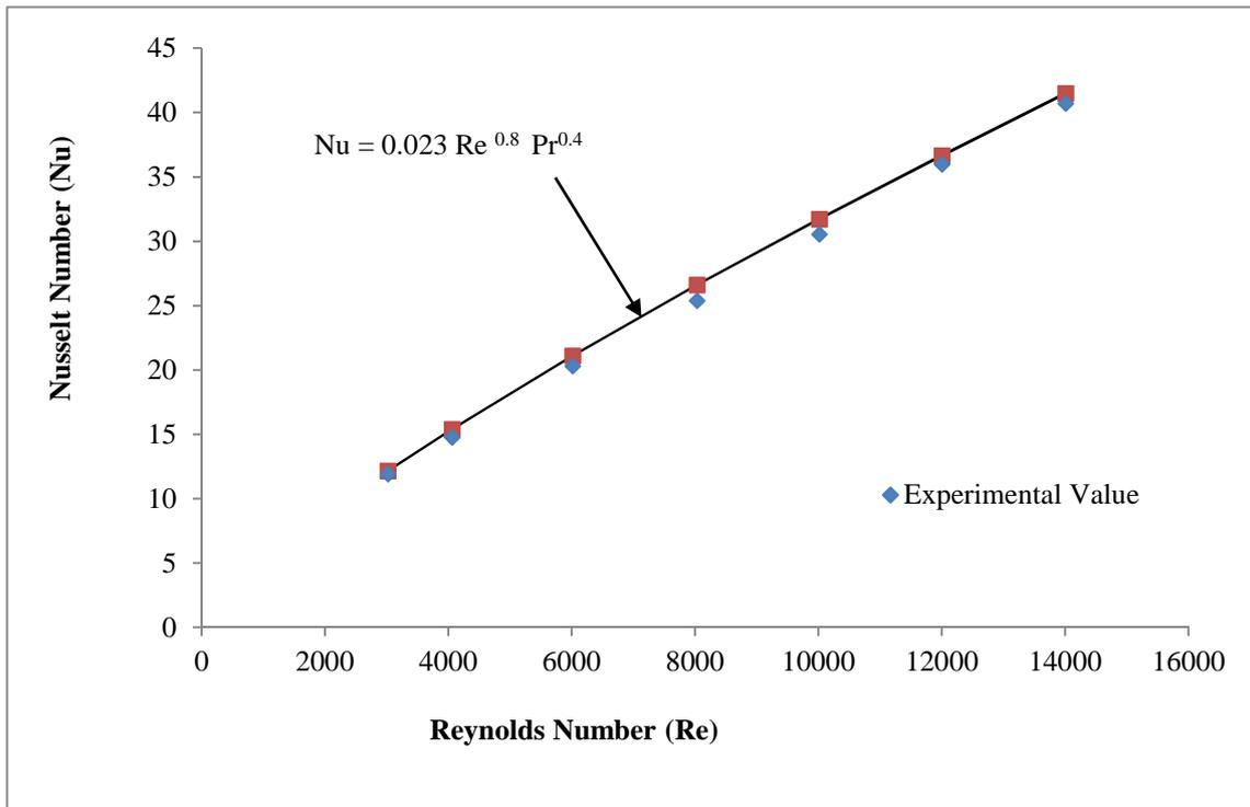
Figure (4) Comparison of experimental and estimated values of Nusselt number of smooth duct.
