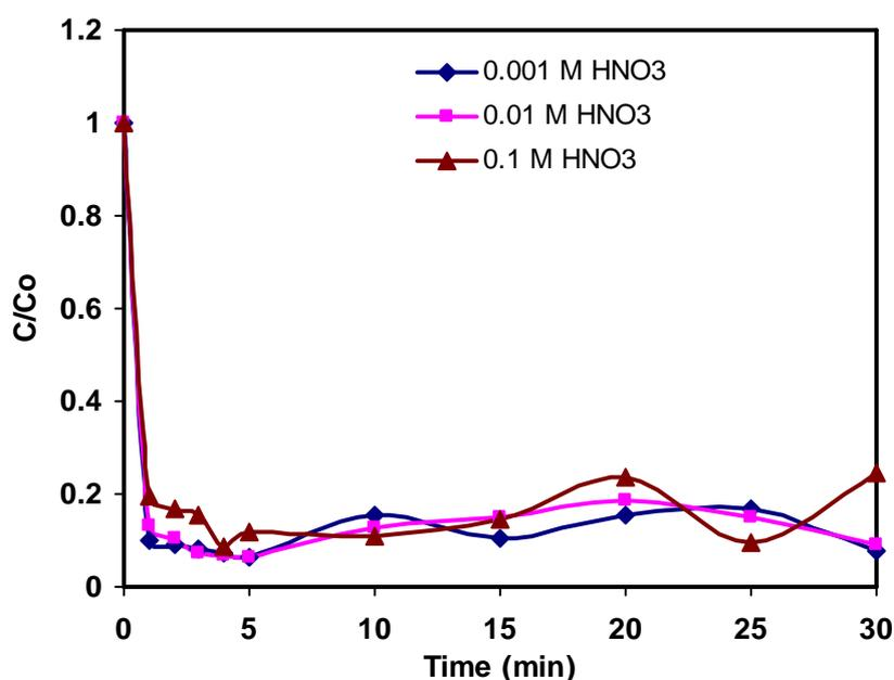
**Fig 2:** Extraction of DCF using 2 w/v % D2EHPA, 2 w/v % Span 80, homogenizer speed 6500 rpm and stirring speed 300rpm at different concentration of stripping phase.
