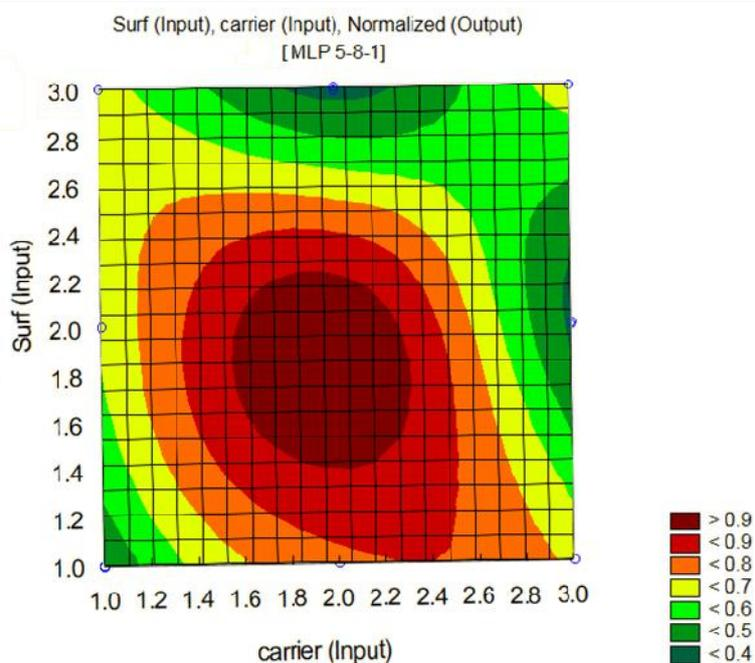
**Fig 5: Combine effect of carrier and surfactant concentration on percentage extraction of DCF.**
