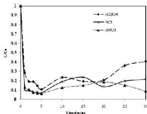
**Fig 1:** Extraction of DCF using 2 w/v % D2EHPA, 2 w/v % Span 80, homogenizer speed 6500 rpm and stirring speed 300rpm with stripping phase concentration of 0.01 M .
