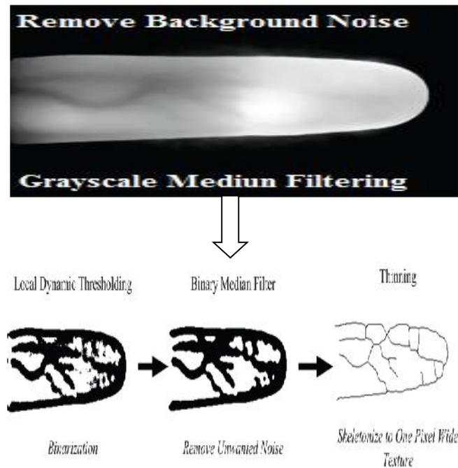
**Figure:-11** Output image of image processing
