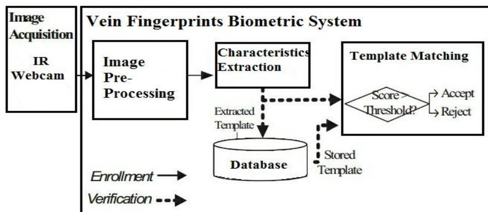
**Figure:-6 Conceptual design of proposed biometric system**
