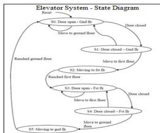
**Figure:-3 Proposed flow diagram of elevator unit**
