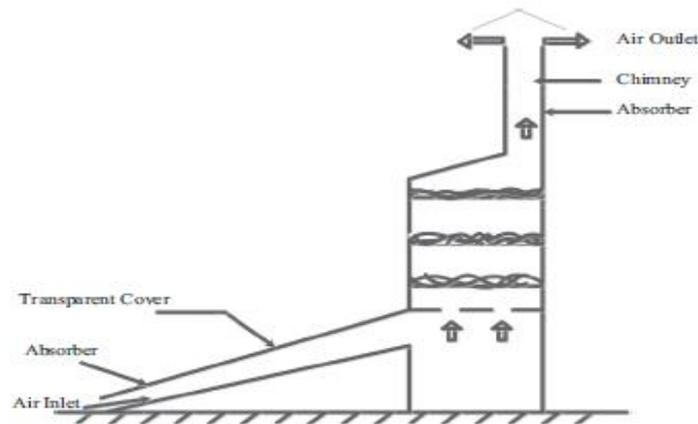
Fig 2. Indirect solar dryer [77]
