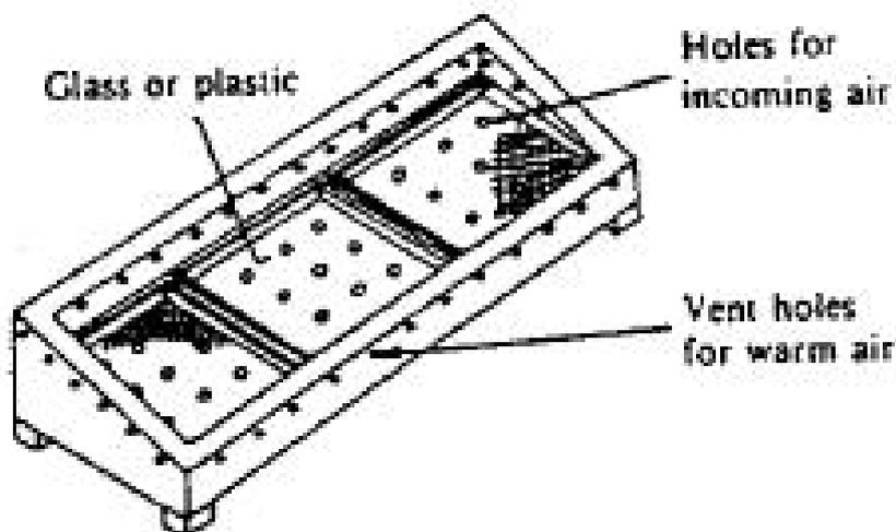
Fig 1. Direct solar dryer [76]
