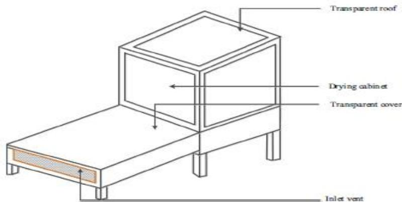
Fig 3. Mixed mode solar dryer [77]
