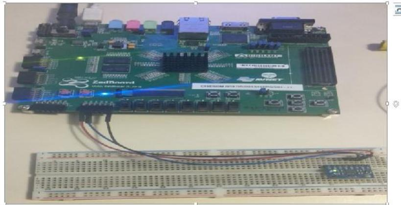
**Fig. 5 I2C Interface of MPU 6050 with ZED Board**
