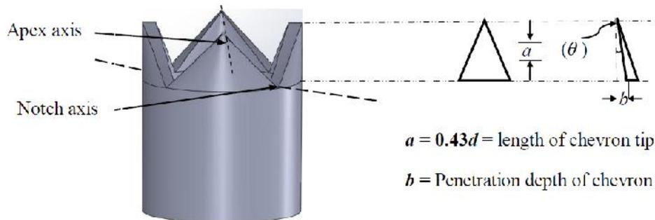
**Figure 2: Geometry of chevron nozzle**
