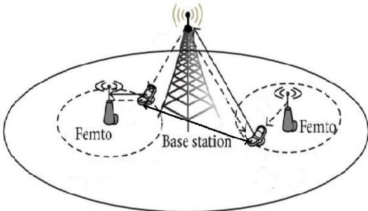
**Fig 1: User equipments communication between Femto and Macro base stations.**
