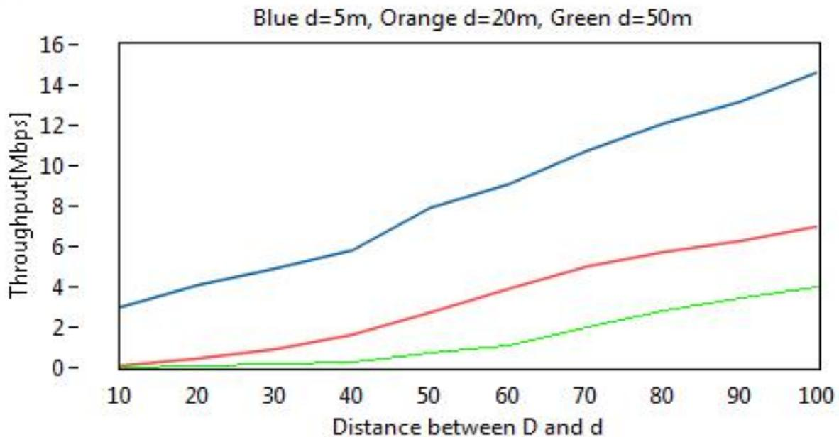
**Fig 3: Macro and Femto users throughput according to  $D$  and  $d$  (Proposed)**
