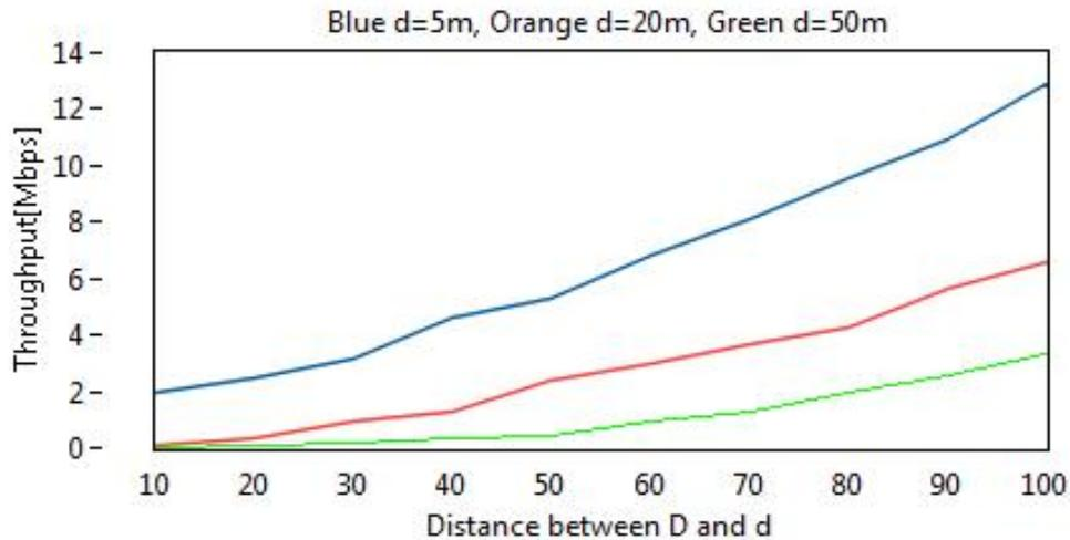
**Fig 2: Macro and Femto users throughput according to  $D$  and  $d$  (Conventional)**
